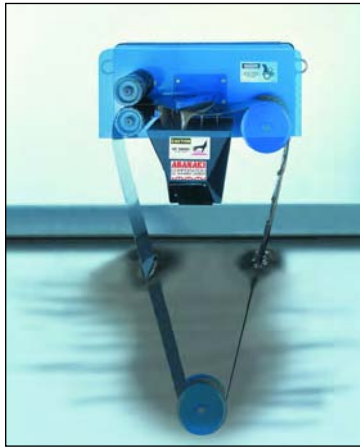
Figure 1. Belt skimmer removing grease from a wastewater sump.
