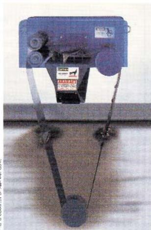
Figure 3. Various pulley assembly designs help improve oil removal by stabilizing a skimmer belt in turbulent fluid.
