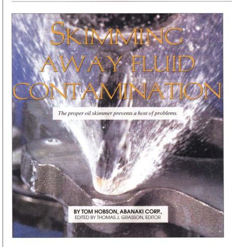
achine coolant or cutting fluid contaminated with tramp oil causes major problems. For instance, contamination reduces fluid life and deteriorates the quality of machined parts. As the problem worsens, the tramp oil accelerates bacterial growth, and the cutting fluid eventually produces a rotten-egg odor. But more detrimental is bacteria-contaminated coolant causing dermatitis.
