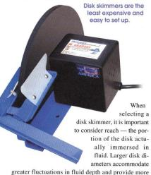
surface area for oil collection. Since the skimmer mounting and disk diameter are fixed, the system collects progressively less oil as the fluid level drops.
